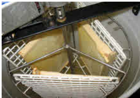
As the frames turn anti-clockwise in this tangential extractor, the honey will be thrown out as the cells are slightly tilted upwards.
